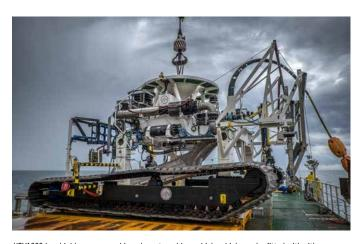
UTV1200 is a highly manoeuvrable subsea trenching vehicle which can be fitted with either a jetting installation or a mechanical chain cutter. Designed to work far from the trenching support vessel, the UTV1200 is capable of excursions of up to 1,500 m from its launch point. Whilst the vehicle concept is very suited to burry array cables, the guaranteed minimum bend radius of 4 m allows UTV1200 to trench large export cables as well with a maximum outer diameter of 300 mm.
