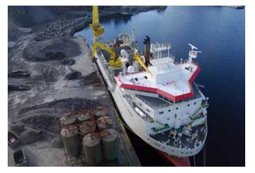
In the Subsea Rock Installation mode, the vessel can install approx. 4,750 t of rock in a single load by means of the excavator, conveyor belt and the fall pipe for accurate rock installation at up to 600 m water depth. Alternatively the rock can be handled through an inclined fall pipe, for secure installation against offshore structures such as jacket platforms, gravity bases or monopile foundations.
