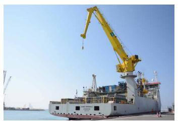
In the Subsea Rock Installation mode, the vessel can install approx. 4,750 t of rock in a single load by means of the excavator, conveyor belt and the fall pipe for accurate rock installation at up to 600 m water depth. Alternatively the rock can be handled through an inclined fall pipe, for secure installation against offshore structures such as jacket platforms, gravity bases or monopile foundations.
