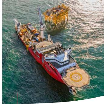
The cable installation vessel Connector connected the cables to substation 'Noord', about 34 km off the coast.
