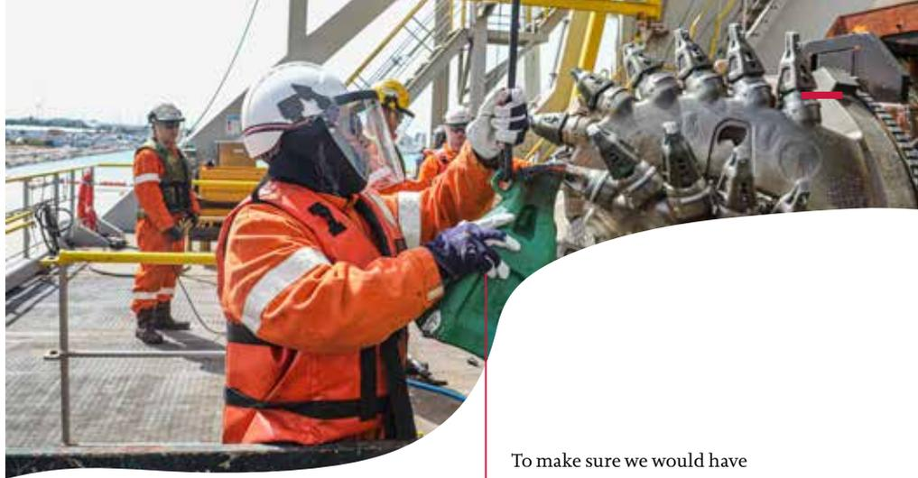
To make sure we would have enough spare parts on site, we pre-mobilised 15,000 cutter teeth and 13 cutter heads. We also set up two mobile welding stations on shore for servicing and repairing the cutter teeth.
