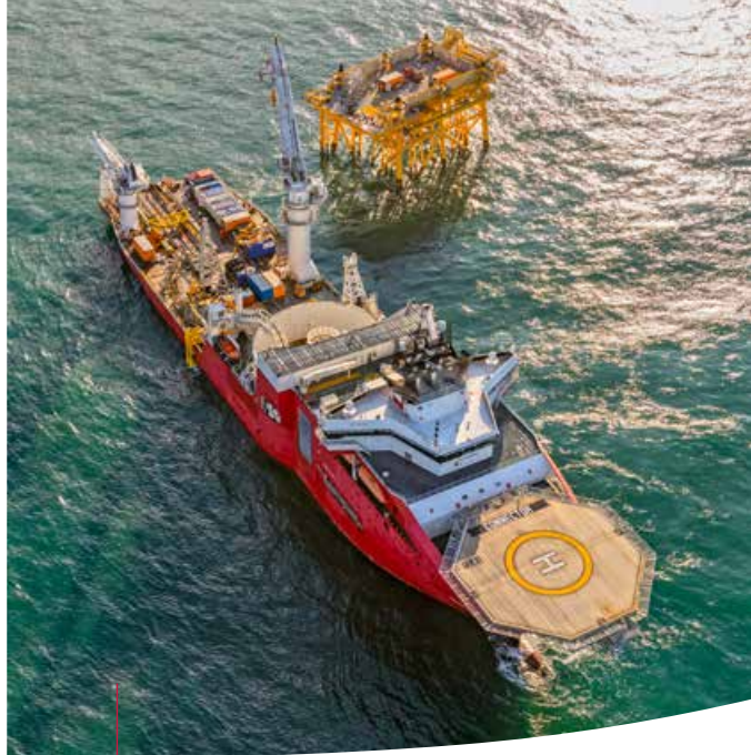
The cable installation vessel Connector connected the cables to substation 'Noord', about 34 km off the coast.
